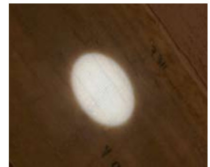
Detail of the Shasthansa quadrant with the pinhole image of the sun at noon
